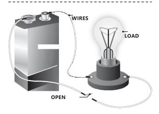
An **open circuit** has a break in the path. There is no flow of
