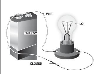
A **closed circuit** is a complete path allowing electricity to flow from the energy source to the load.
